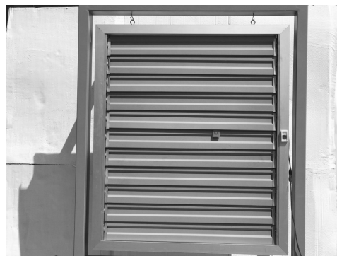
Figure 12. Mock-up stand for hanging the prototype of an automatically adjustable sun louvers.
