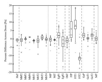
Figure 1. The boxplots present the measurement results of differential pressure across the automatic entrance doors.
