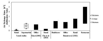
Figure 7. Calculated air exchange rates of air infiltration in retails and supermarkets compared to three existing studies.
