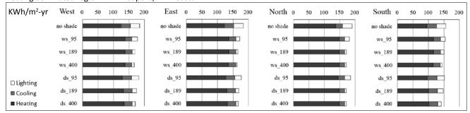
Figure 4. Results for perimeter offices with roller shades on insulated low-E glazing (window A) using different solar control strategies and daylight dimming control.
