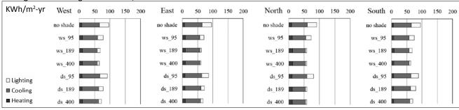
Figure 5. Results for perimeter offices with roller shades on insulated low-E glazing (window B) using different solar control strategies and daylight dimming control.
