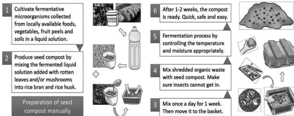
Figure 2. Process of Takakura Composting Method (TCM). Source: Maeda (2009) modified by authors
