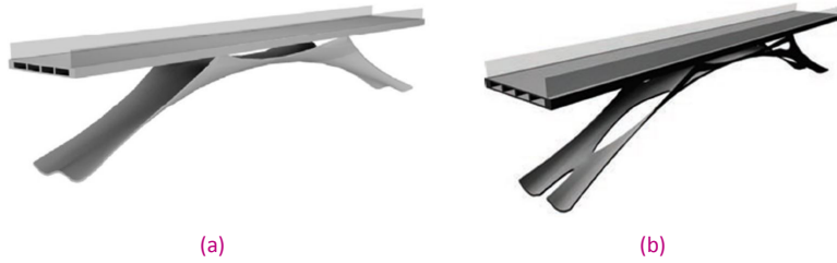
Figure 18. (a) Model of shell-supported bridge (Briseghella et al., 2013). (b) Model of shell-supported bridge with cavity insertion (Briseghella et al., 2013).
