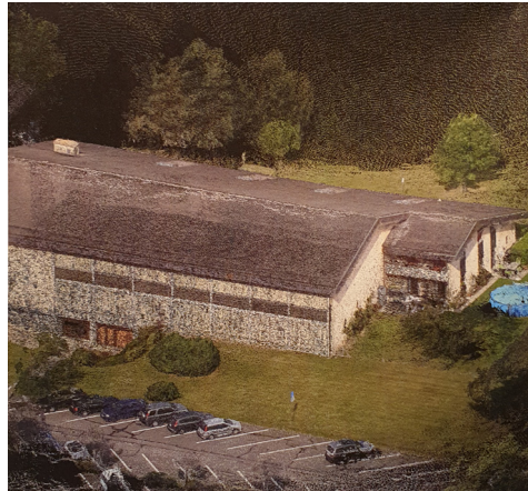
Figure 1. Point cloud of a building showing mapping results of oblique imagery© Pix4D (Source: Calvo, 2015, p.28)
