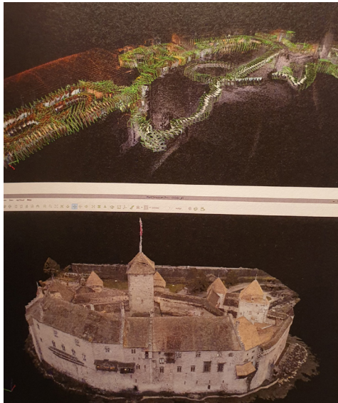
Figure 2. 3D point cloud view of Chillon Castle's lake-side.© Pix4D (Source: Calvo, 2015, p.67)
