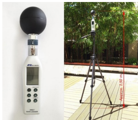
Figure 5 WGBT Data Logger AD-5695DL and the setting
