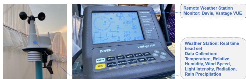
Figure 3. Weather station set for outdoor monitoring, Supatra Melon Farm, Saraburi.
