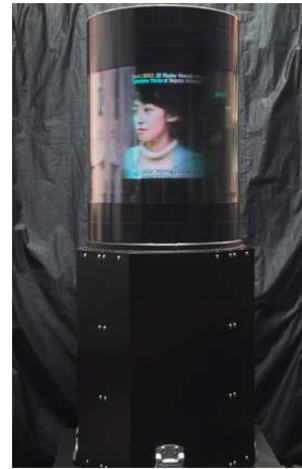
Fig.25: The SeeLINDER, a 360 degree, ray-reproducing display
