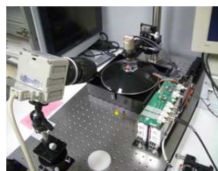
Fig.22: Mirror-scan ray capturing system
