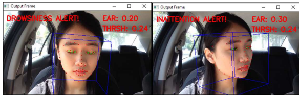
Fig.14: Detection results (left) drowsiness alert and (right) inattention alert.
