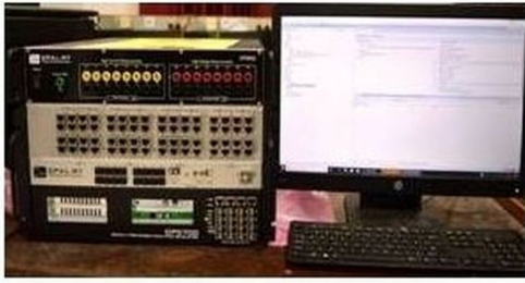
Fig.20: Experimental setup based on OPAL-RT.
