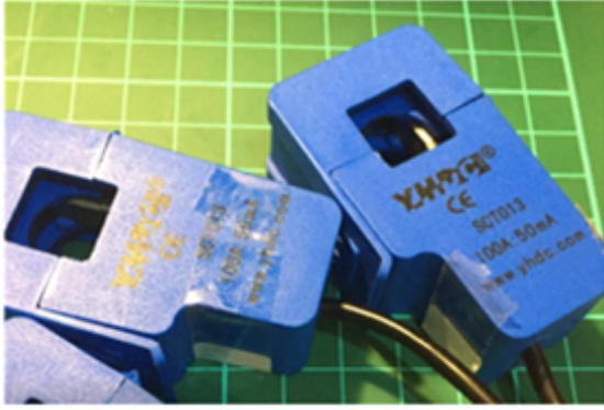
Fig.4: Current transformers for the prototype instrument.
