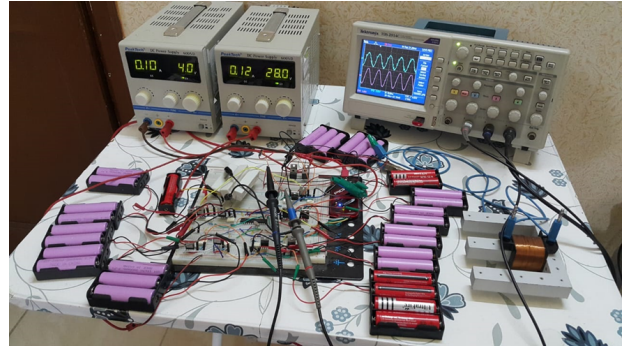
Fig. 13: Experimental setup of the single phase 15 levels MLI.
