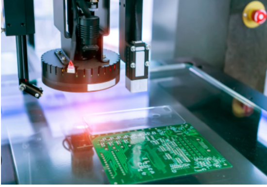
Fig. 3: Automated Optical Inspection (AOI) [5].
