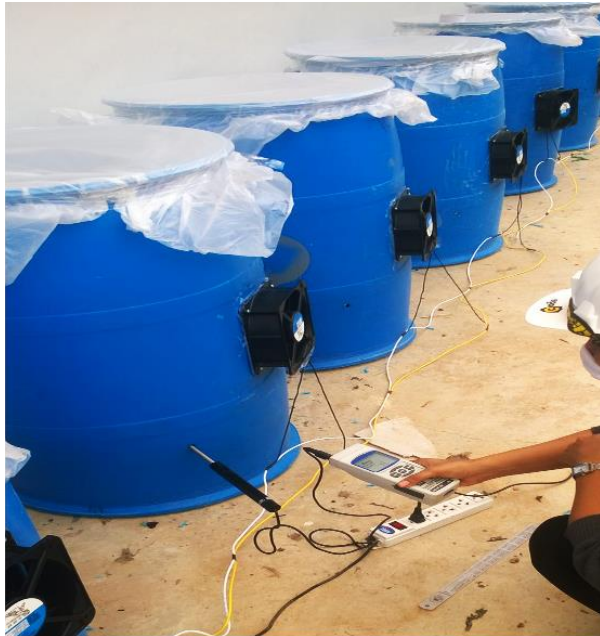
Fig. 3 How to measure the characteristics of MSW outside the experimental plastic drum
