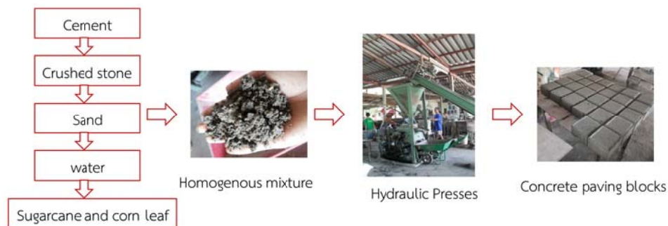
Fig. 1 Schematic diagram of preparation for Paver blocks containing Sugarcane and Corn Leaf.
