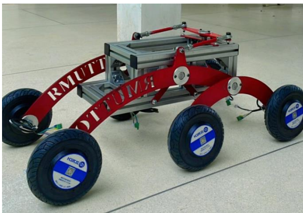
Fig. 9 Prototype of an explorer robot by using rocker-bogie suspension
