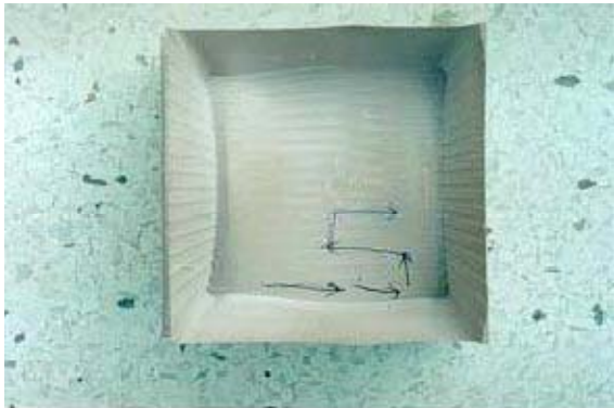
Fig.14: The real cut of the saddle surface using the proposed algorithms
