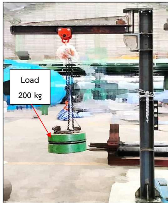
Figure 9 Shows the Type-3 Jib Crane; The actual load testing.
