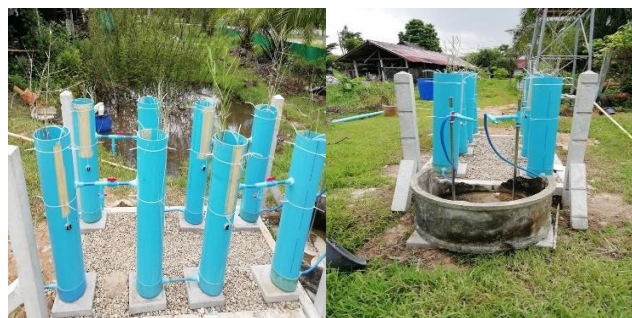
Figure 1: Planted constructed wetland showing 2 systems with 4 cylinders each
