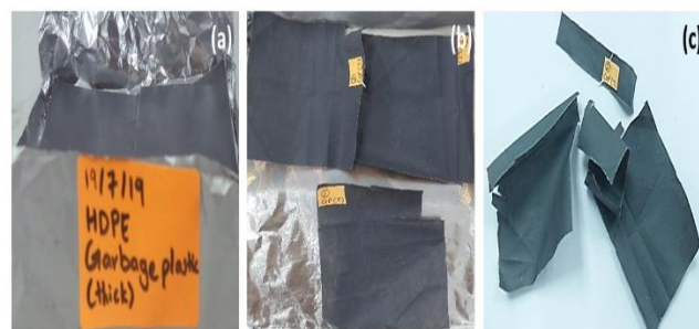
Figure 2. (a) The HDPE sheet (control), (b) The HDPE sheet after 15 days of UV treatment, (c) The HDPE sheet after 30 days of UV treatment
