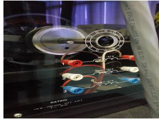
Figure 3 Squirrel cage induction motor.
