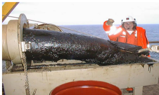
Figure 6 Wax plug in wellbore on platform C in the North Sea (Zhu et al., 2008).
