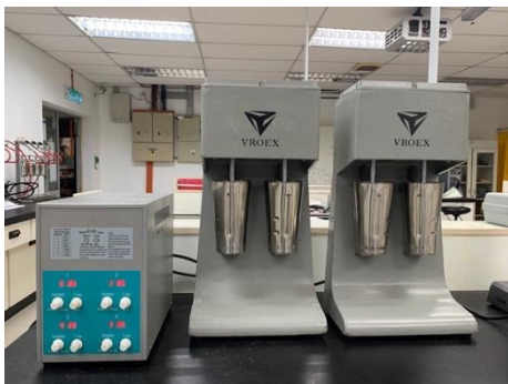
Figure 1 Mud mixer for the mixing of WBDM.
