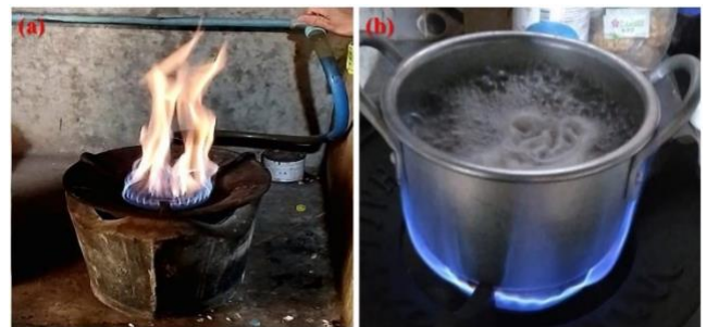
Figure 4. Balloon biogas pilot model installation with productive application (a) burning test and (b) making hot water
