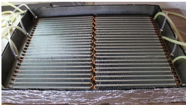
Figure 6. Setup 3 where condensers are in series
