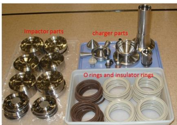
Figure 2 Impactor stages and charger parts of the ELPI+ instruments
