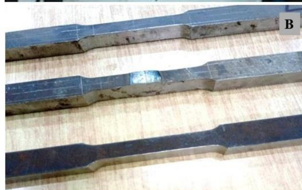
Figure 6. Tensile testing setup for API X70 steel: (A) UTM for tensile tests per ASTM E8/E8M standards and (B) Standard tensile specimens from weld zone, HAZ, and parent material of steel plate
