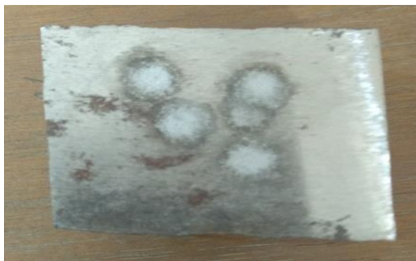
Figure 2. Surface of API X70 steel sample after chemical and spectroscopic analysis
