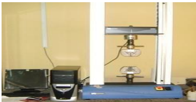
Figure 8. Computerized Instron Universal Testing Machine used for compression testing
