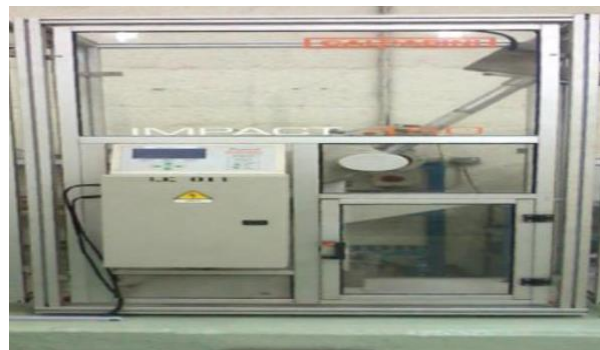
Figure 7. Charpy impact testing machine used for toughness evaluation
