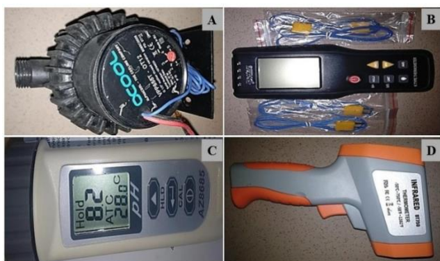
Figure 1. Water circulation pump (A), digital thermometer (B), digital pH meter (C), and IR thermometer (D) are used in the corrosion rig to help collect the necessary data.
