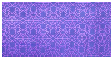
(b) Result of actual weaving using the design technique to obtain the pattern of wallpaper group P6m
