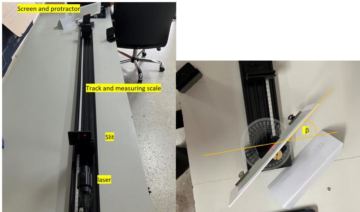
Figure 2. The picture shows the experiment setup. Laser, slit, and screen are placed on a track with a measuring scale. A protractor is used for measuring the screen angle \beta .
