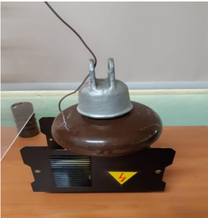
Figure 8 Flashover experiment of insulator
