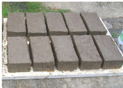
Figure 5 Adobe bricks formed by pouring clay into a mold and compacting it with foot pressure
