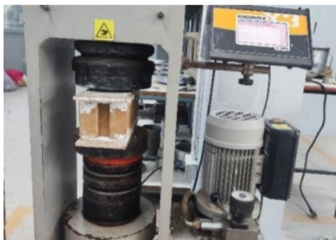
Fig. 4 Compressive strength test of interlocking block
