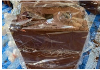
Fig. 3 Curing interlocking block with plastic bags
