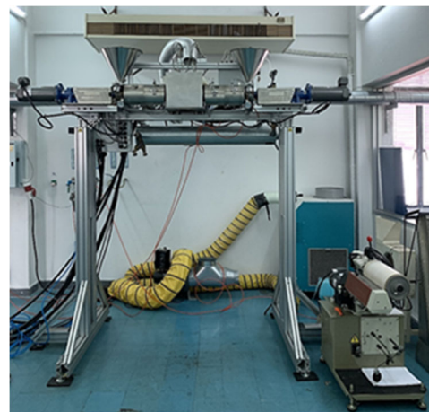
Fig. 1 Lab scale bicomponent extruder fed spinning machine model LBS-100, Hills, Inc.
