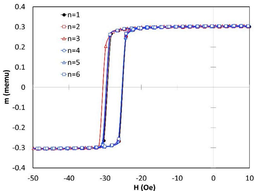
Figure 1 n<sup>th</sup> m-H curves of the Ni<sub>81</sub>Fe<sub>19</sub>/Ir<sub>20</sub>Mn<sub>80</sub> exchange-biased thin films, where n=1 to 6.
