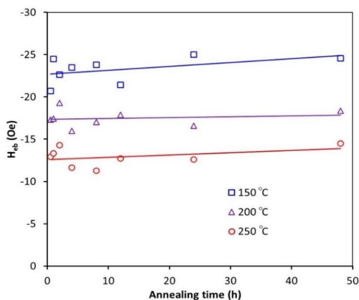
**Figure 5** Exchange bias field of the samples annealed with different annealing times in argon atmosphere.
