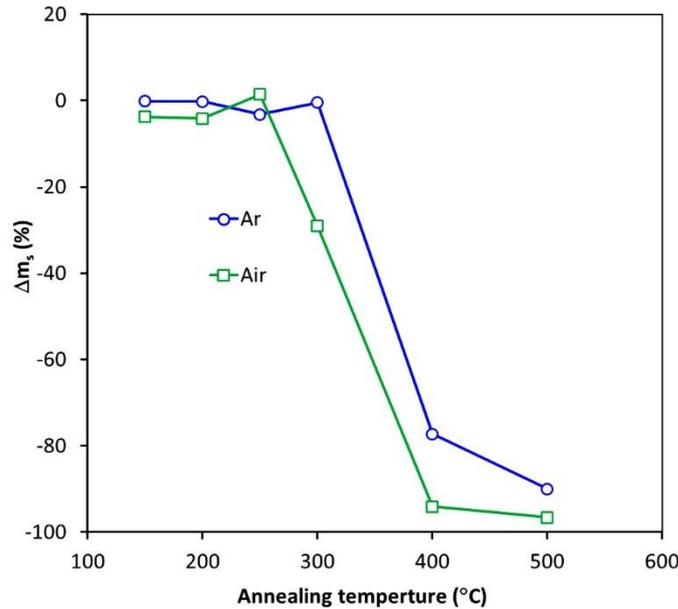
**Figure 3** Percentage decrease of the saturation magnetic moment ( $m_s$ ) of the samples annealed at different temperatures in argon atmosphere compared with those of the samples annealed in air atmosphere.
