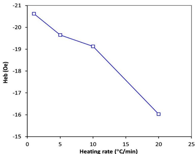
**Figure 7** Exchange bias field of the samples annealed at 200 °C in an argon atmosphere with different heating rates.
