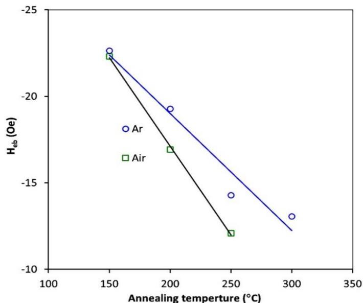
**Figure 4** Variation of exchange bias field of the samples annealed at different temperatures in argon atmosphere compared with those of the samples annealed in air atmosphere.
