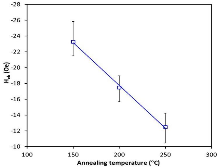
**Figure 6** Average exchange bias field of the samples annealed at different temperatures in an argon atmosphere.
