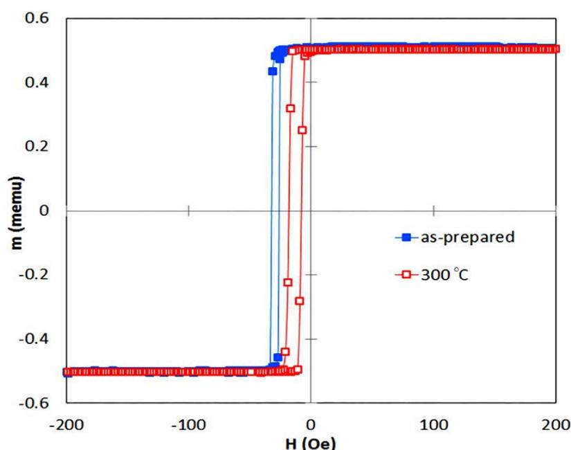
**Figure 2** m-H curves of the sample annealed at 300 °C in argon atmosphere for 2 h with a heating rate of 5 °C/min compared with that of the as-prepared sample.
