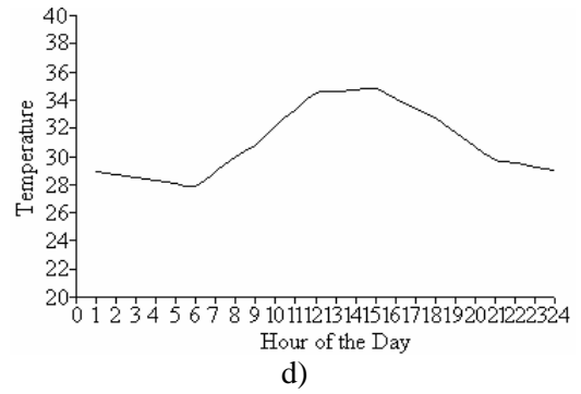
Figure7. Inputs for the building thermal model (a) Occupancy (b) Light-ing (c) Equipment (d) Outside air temperature
