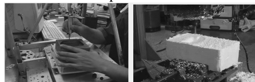
The master arm with force reflection
