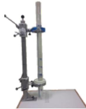
Fig. 3. The egg-drop test apparatus.
