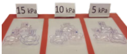
Fig. 2. TPU with air filled 5, 10 and 15 kPa and ironing the air pathway to close the system.
