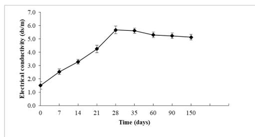
**Fig. 2.** Illustration of bio-extract electrical conductivity (EC) during 5 months of fermentation.
