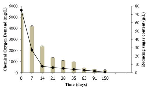
**Fig. 3.** Change in chemical oxygen demand (mg L<sup>-1</sup>) (line graph) and reducing sugar content (g L<sup>-1</sup>) (bar chart) in bio-extract during 150 days of fermentation.
