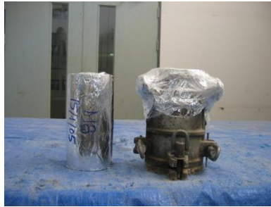
Fig. 3. Specimen covered by foil and plastic sheet.
