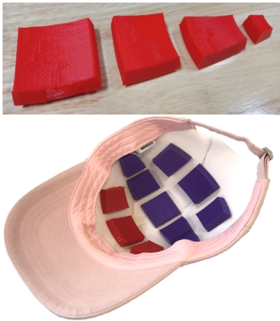
Fig. 29. The fabricated prototype of paddings and the foldable hat insert when assembled with the baseball cap.
