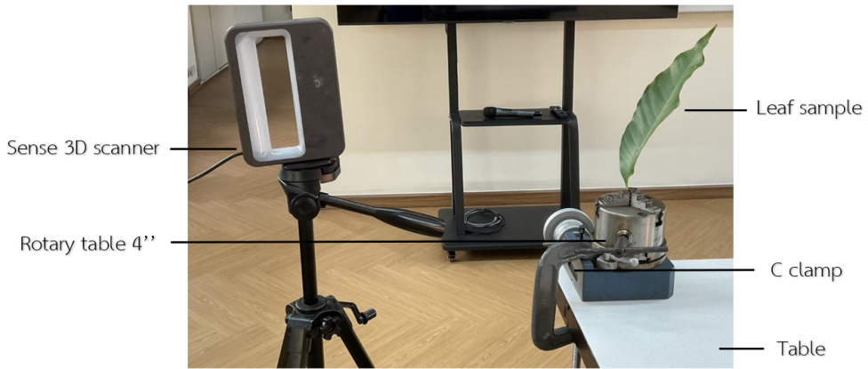
Fig. 2. Setup of the scanning apparatus.
