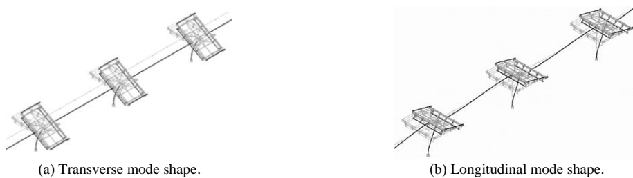
Fig. 7. Fundamental modes of vibration of the studied bridges in transverse and longitudinal directions.
