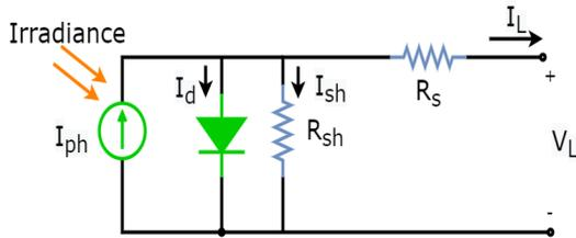
Fig. 1. Single diode circuit of PV [30].
