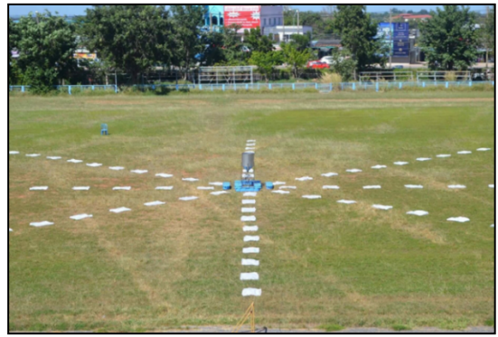
Fig. 7. Collecting experimental results of the giant freshwater prawn feeder.
