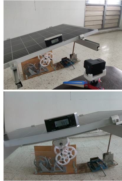
Fig. 4. Isometric view (up) and camera view (down) of the test setup for the presented system using a <0.10^\circ accuracy digital protractor and a GoPro 7 Black set to 120 frames per second.
