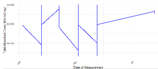
Fig. 10. Fluctuation of total absorbed radiation dose over time in the vicinity of the Chernobyl Nuclear Power Plant (ChNPP).
