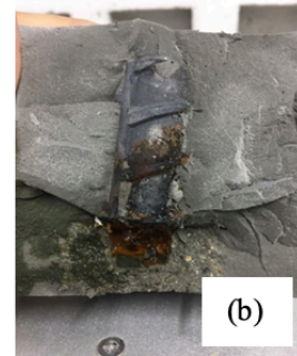
Fig. 6. Testing of chloride migration in a non-steady state for the RRPC facility: (a) Specimens during testing and (b) Split specimen after testing.
