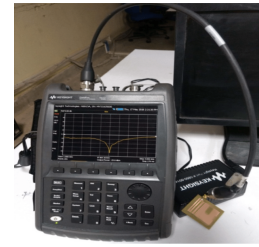
Fig. 8. Experimental setup of the UHF 432.5 MHz microstrip rampart line antenna measured by antenna testing spectrum analyzer.
