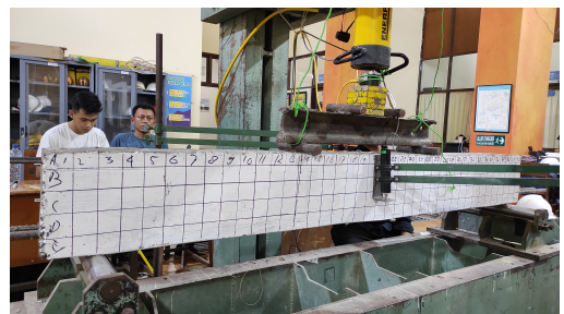
Fig. 5. Testing process of the splice beam.
